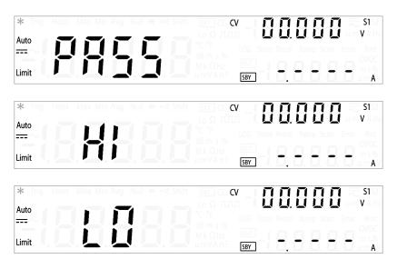
Each time the input value transitions from "PASS" to "HI" or from "PASS" to "LO", or when transitioning directly from "HI" to "LO" or "LO" to "HI", the instrument beeps once (if the beeper is enabled).
