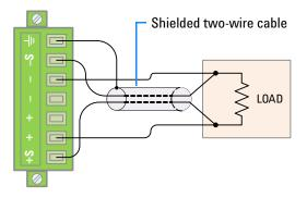
Figure 3-3 Remote sensing connections
