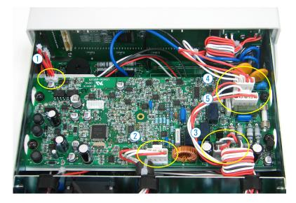
8 Remove the top layer circuit board. Loosen the four captive screws in the top layer circuit board and remove the top layer circuit board. Remove the protective metal sheet as well.
