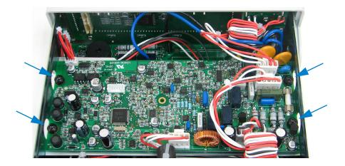
**9** Disconnect the individual wires from the bottom layer circuit board as shown below.
