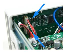
**c** Disconnect the individual wires from the top layer circuit board as shown below.
