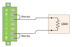
Figure 3-4 Local sensing connections
