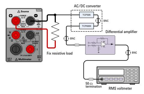
Figure 5-11 Test setup for CC noise effect verification
