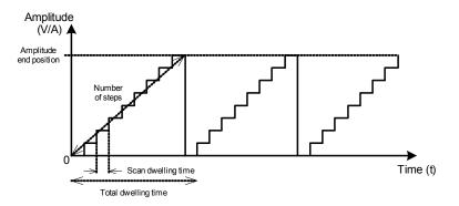
The total dwell time is will increase with respect to the number of steps and the scan dwell time per step selected. The scan dwell time is defined as the length of time the scan signal will "dwell" in the present step before incrementing to the next step.
