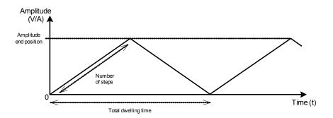
The ramp dwelling time will be set to the fastest of the instrument capability (typically ~300 ms per step). A higher number of steps provides a more linear ramp signal. This however will result in an increase in the total dwelling time. A lower number of steps will result in a shorter total dwelling time and a more stepped ramp signal.
