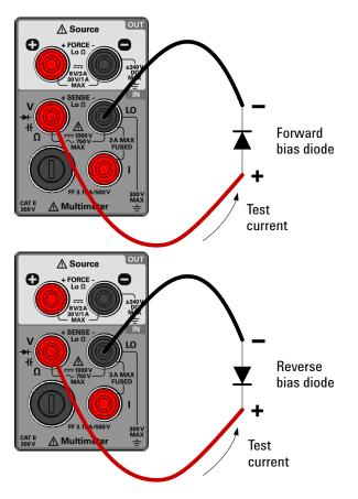
Figure 2-9 Terminal connections for diode tests
