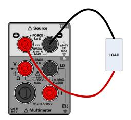
Figure 3-1 Constant voltage mode terminal connections
