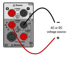
Figure 2-1 Terminal connections for voltage measurements
