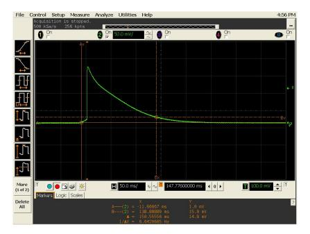
Figure 5-13 Load transient response time
