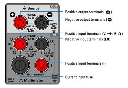
Figure 1-7 U3606A connector terminals
