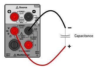
Figure 2-7 Terminal connections for capacitance measurements
