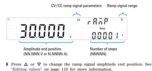
7 Press I or I until the cursor is position on the ramp signal number of steps. Press I or I to change the number of steps for the ramp signal to increment from zero to the amplitude end position. See "Editing values" on page 110 for more information.
