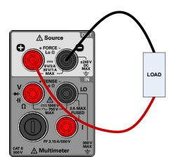
Figure 3-2 Constant current mode terminal connections
