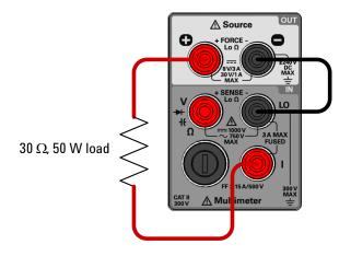
**9** Verify the constant current adjustments using the "CC programming and readback accuracy" on page 163.
