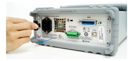
2 Remove the fuse holder assembly from the rear panel.
