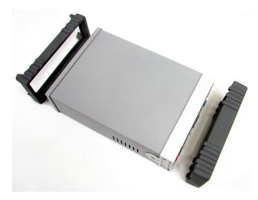
**4 Remove the rear bezel.** Loosen the two captive screws in the rear bezel and remove the rear bezel.
