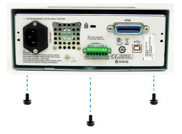
**5 Remove the cover.** Remove the screws in the bottom of the cover.
