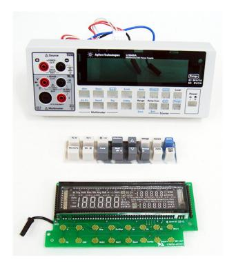
**13 Remove the keypad and display assembly.** The rubber keypad and VFD display assembly can now be pulled out from the plastic housing.
