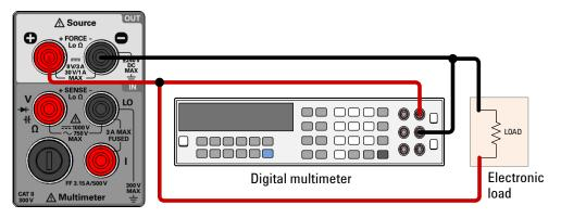
Figure 5-6 Test setup for CV load and line regulation verification
