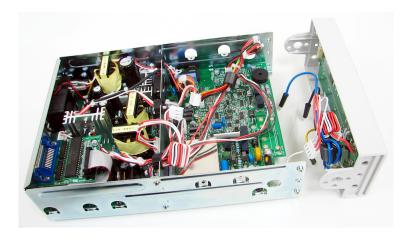
**11** You can now pry the side of the front panel from the chassis and remove it.
