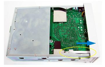
**b** Disconnect the two ribbon cable connectors from the front panel.
