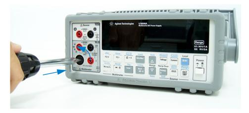
**2** Turn the screwdriver anti-clockwise to remove the fuse holder assembly from the front panel.
