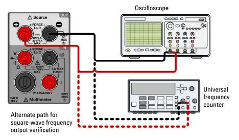
Figure 5-12 Test setup for square-wave output verification
