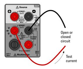
Figure 2-8 Terminal connections for continuity tests
