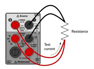
Figure 2-4 Terminal connections for 4-wire resistance measurements
