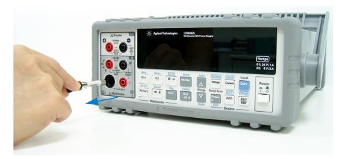
**3** Remove the faulty current input fuse and replace a new current input fuse into the fuse holder assembly.
