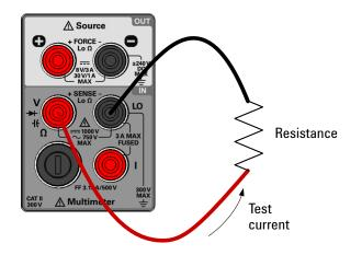
Figure 2-3 Terminal connections for 2-wire resistance measurements
