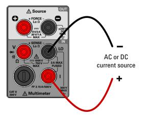
Figure 2-2 Terminal connections for current measurements
