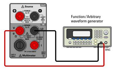
Figure 5-4 Test setup for frequency gain verification
