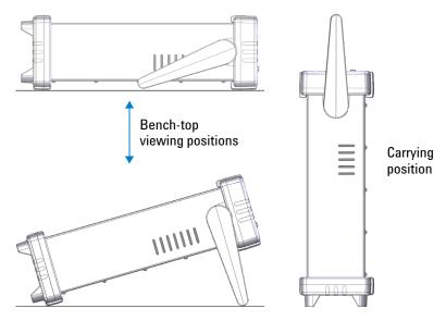
Figure 1-1 U3606A handle adjustments
