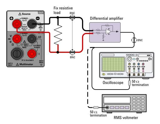
Figure 5-7 Test setup for CV noise effect verification
