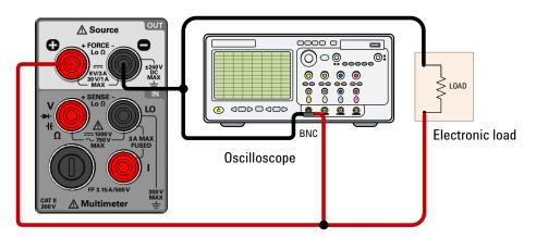
Figure 5-8 Test setup for load transient response time verification
