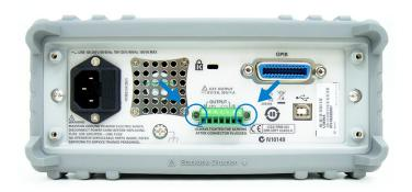
**3** Gently pull the rear output terminal block out.
